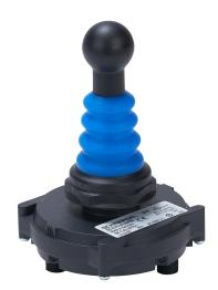
Schmersal selector switch, IP65, IP67, IP69 and IP69K, 22mm, 4-position, momentary, (8) N.O. contact(s), plastic base, plastic bezel, Operator: blue, joystick, 25mm, round, plastic.
