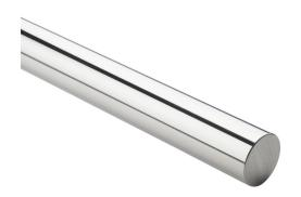
PBC Simplicity 60 Plus series linear precision ground round shaft, 440C stainless steel, RC50-55, 8-12Ra, 1-1/4in diameter, 36in length. For use with 1-1/4in PBC bearings.
