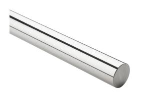
PBC Simplicity 60 Plus series linear precision ground round shaft, 440C stainless steel, RC50-55, 8-12Ra, 1-1/4in diameter, 24in length. For use with 1-1/4in PBC bearings.
