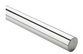
PBC Simplicity 60 Plus series linear precision ground round shaft, 1060 steel, RC60-65, 8-12Ra, 1-1/4in diameter, 36in length. For use with 1-1/4in PBC bearings.
