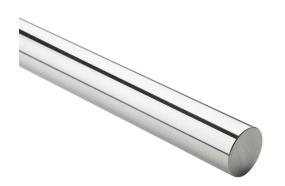
PBC Simplicity 60 Plus series linear precision ground round shaft, 1060 steel, RC60-65, 8-12Ra, 1-1/4in diameter, 24in length. For use with 1-1/4in PBC bearings.
