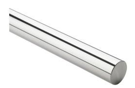
PBC Simplicity 60 Plus series linear precision ground round shaft, 1060 steel, RC60-65, 8-12Ra, 1-1/4in diameter, 12in length. For use with 1-1/4in PBC bearings.
