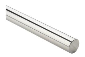
PBC Simplicity 60 Plus series linear precision ground round shaft, 440C stainless steel, RC50-55, 8-12Ra, 1in diameter, 24in length. For use with 1in PBC bearings.
