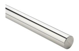
PBC Simplicity 60 Plus series linear precision ground round shaft, 1060 steel, RC60-65, 8-12Ra, 1in diameter, 36in length. For use with 1in PBC bearings.
