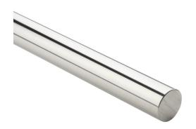
PBC Simplicity 60 Plus series linear precision ground round shaft, 1060 steel, RC60-65, 8-12Ra, 1in diameter, 12in length. For use with 1in PBC bearings.
