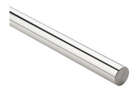
PBC Simplicity 60 Plus series linear precision ground round shaft, 440C stainless steel, RC50-55, 8-12Ra, 3/4in diameter, 36in length. For use with 3/4in PBC bearings.
