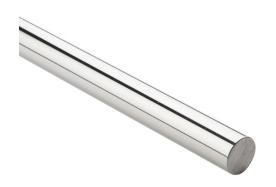
PBC Simplicity 60 Plus series linear precision ground round shaft, 440C stainless steel, RC50-55, 8-12Ra, 3/4in diameter, 12in length. For use with 3/4in PBC bearings.
