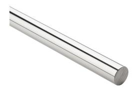
PBC Simplicity 60 Plus series linear precision ground round shaft, 1060 steel, RC60-65, 8-12Ra, 3/4in diameter, 36in length. For use with 3/4in PBC bearings.
