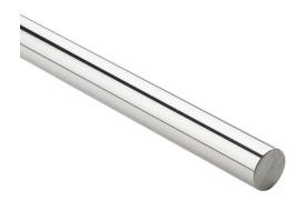
PBC Simplicity 60 Plus series linear precision ground round shaft, 1060 steel, RC60-65, 8-12Ra, 3/4in diameter, 24in length. For use with 3/4in PBC bearings.
