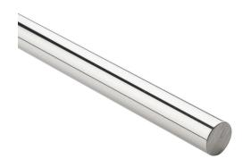
PBC Simplicity 60 Plus series linear precision ground round shaft, 1060 steel, RC60-65, 8-12Ra, 3/4in diameter, 12in length. For use with 3/4in PBC bearings.
