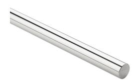
PBC Simplicity 60 Plus series linear precision ground round shaft, 440C stainless steel, RC50-55, 8-12Ra, 5/8in diameter, 36in length. For use with 5/8in PBC bearings.
