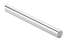
PBC Simplicity 60 Plus series linear precision ground round shaft, 440C stainless steel, RC50-55, 8-12Ra, 5/8in diameter, 24in length. For use with 5/8in PBC bearings.
