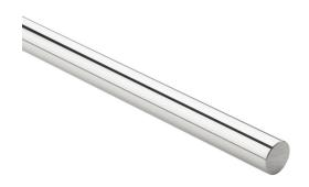
PBC Simplicity 60 Plus series linear precision ground round shaft, 440C stainless steel, RC50-55, 8-12Ra, 5/8in diameter, 12in length. For use with 5/8in PBC bearings.
