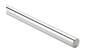
PBC Simplicity 60 Plus series linear precision ground round shaft, 1060 steel, RC60-65, 8-12Ra, 5/8in diameter, 24in length. For use with 5/8in PBC bearings.
