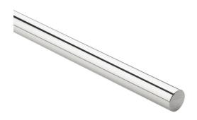
PBC Simplicity 60 Plus series linear precision ground round shaft, 1060 steel, RC60-65, 8-12Ra, 5/8in diameter, 12in length. For use with 5/8in PBC bearings.
