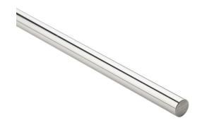
PBC Simplicity 60 Plus series linear precision ground round shaft, 440C stainless steel, RC50-55, 8-12Ra, 1/2in diameter, 36in length. For use with 1/2in PBC bearings.
