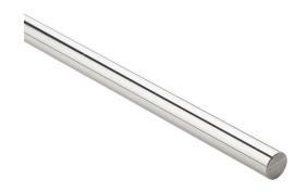
PBC Simplicity 60 Plus series linear precision ground round shaft, 440C stainless steel, RC50-55, 8-12Ra, 1/2in diameter, 24in length. For use with 1/2in PBC bearings.
