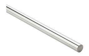
PBC Simplicity 60 Plus series linear precision ground round shaft, 440C stainless steel, RC50-55, 8-12Ra, 1/2in diameter, 12in length. For use with 1/2in PBC bearings.
