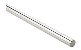
PBC Simplicity 60 Plus series linear precision ground round shaft, 1060 steel, RC60-65, 8-12Ra, 1/2in diameter, 36in length. For use with 1/2in PBC bearings.
