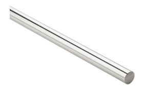
PBC Simplicity 60 Plus series linear precision ground round shaft, 1060 steel, RC60-65, 8-12Ra, 1/2in diameter, 24in length. For use with 1/2in PBC bearings.
