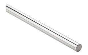
PBC Simplicity 60 Plus series linear precision ground round shaft, 1060 steel, RC60-65, 8-12Ra, 1/2in diameter, 12in length. For use with 1/2in PBC bearings.
