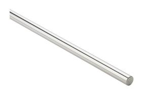
PBC Simplicity 60 Plus series linear precision ground round shaft, 440C stainless steel, RC50-55, 8-12Ra, 3/8in diameter, 12in length. For use with 3/8in PBC bearings.
