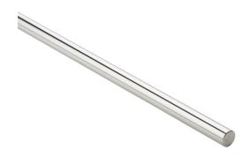
PBC Simplicity 60 Plus series linear precision ground round shaft, 1060 steel, RC60-65, 8-12Ra, 3/8in diameter, 18in length. For use with 3/8in PBC bearings.
