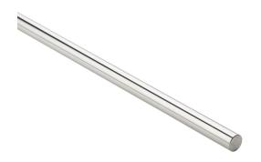
PBC Simplicity 60 Plus series linear precision ground round shaft, 1060 steel, RC60-65, 8-12Ra, 3/8in diameter, 12in length. For use with 3/8in PBC bearings.
