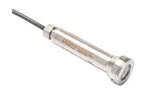
ProSense hydrostatic submersible level transmitter, 0 to 30 psig (69.2ft of water column) sensing range, 4-20 mA, 1.26in diameter housing, shielded and vented 100ft cable, hazardous location rated.
