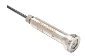
ProSense hydrostatic submersible level transmitter, 0 to 20 psig (46.1ft of water column) sensing range, 4-20 mA, 1.26in diameter housing, shielded and vented 60ft cable, hazardous location rated.
