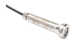
ProSense hydrostatic submersible level transmitter, 0 to 10 psig (23.1ft of water column) sensing range, 4-20 mA, 1.26in diameter housing, shielded and vented 40ft cable, hazardous location rated.
