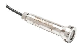
ProSense hydrostatic submersible level transmitter, 0 to 5 psig (11.5ft of water column) sensing range, 4-20 mA, 1.26in diameter housing, shielded and vented 30ft cable, hazardous location rated.
