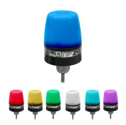
Patlite NE-A series integrated LED audible-visual signal beacon, 88 dB at 1m, continuous/intermittent tone(s), touch to acknowledge, continuous, multi-color, 56mm, 12-24 VDC, IP65.
