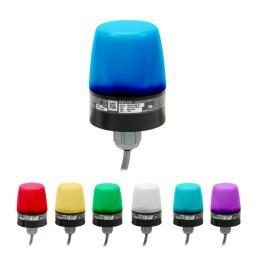
Patlite NE-A series integrated LED audible-visual signal beacon, 88 dB at 1m, continuous/intermittent tone(s), continuous or flashing (500ms), multi-color, 56mm, 12-24 VDC, IP65.
