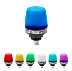
Patlite NE-A series LED industrial signal beacon, 56mm, red/ amber/green/blue/white/cyan/purple, continuous, IP67 and IP69K, direct mount, 12-24 VDC. Requires 5-pin female M12 cable.
