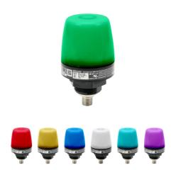
Patlite NE-IL series LED industrial signal beacon, 56mm, red/amber/green/blue/white/cyan/purple, selectable permanent, flashing, double flash or triple flash, IP65, direct mount, touch to acknowledge, 24 VDC, IO-Link Class A Device.
