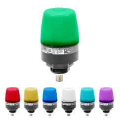
Patlite NE-IL series integrated LED audible-visual signal beacon, 88 dB at 1m, (8) selectable tone(s), touch to acknowledge, selectable permanent, flashing, double flash or triple flash, multicolor, 56mm, 24 VDC, IO-Link Class A Device, IP65.
