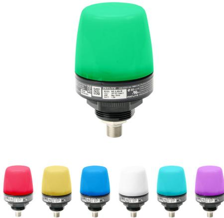
Patlite NE-IL series LED industrial signal beacon, 56mm, red/amber/green/blue/white/cyan/purple, selectable permanent, flashing, double flash or triple flash, IP65, direct mount, 24 VDC, IO-Link Class A Device. Requires 5-pin female M12 cable.
