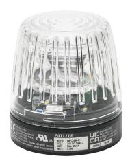
Patlite NE-A series LED industrial signal beacon, 56mm, white, continuous, IP65, direct mount, 24 VDC.
