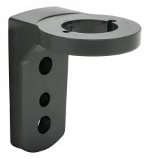
Patlite mounting bracket, wall mount, 56mm diameter, 82mm height, dark gray, polycarbonate. For use with Patlite NE-A and NE-IL series beacons.
