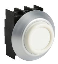
Schmersal pushbutton, IP67 and IP69K, 22mm, momentary, operator only, plastic base, plastic bezel, Operator: white, extended, 27mm, round, plastic. Requires contact blocks.
