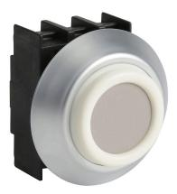
Schmersal pushbutton, IP67 and IP69K, 22mm, momentary, operator only, plastic base, plastic bezel, Operator: gray, extended, 27mm, round, plastic. Requires contact blocks.
