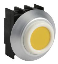
Schmersal pushbutton, IP67 and IP69K, 22mm, momentary, operator only, plastic base, plastic bezel, Operator: yellow, extended, 27mm, round, plastic. Requires contact blocks.
