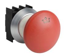
Schmersal emergency stop pushbutton, IP67 and IP69K, 22mm, push to lock, pull to reset, operator only, plastic base, plastic bezel, Operator: red, mushroom, 50mm, round, plastic, operator text "push/pull symbol". Requires contact blocks.
