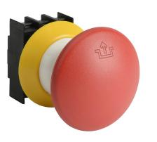
Schmersal emergency stop pushbutton, IP67 and IP69K, 22mm, push to lock, pull to reset, operator only, plastic base, plastic bezel, yellow, Operator: red, mushroom, 50mm, round, plastic, operator text "push/pull symbol". Requires contact blocks.
