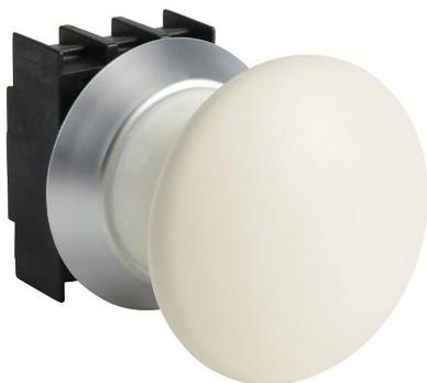
Schmersal pushbutton, IP67 and IP69K, 22mm, momentary, operator only, plastic base, plastic bezel, Operator: white, mushroom, 50mm, round, plastic. Requires contact blocks.
