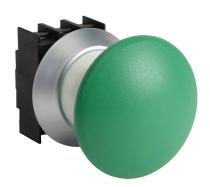
Schmersal pushbutton, IP67 and IP69K, 22mm, momentary, operator only, plastic base, plastic bezel, Operator: green, mushroom, 50mm, round, plastic. Requires contact blocks.
