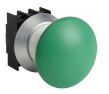
Schmersal pushbutton, IP67 and IP69K, 22mm, momentary, operator only, plastic base, plastic bezel, Operator: green, mushroom, 50mm, round, plastic. Requires contact blocks.
