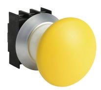
Schmersal pushbutton, IP67 and IP69K, 22mm, momentary, operator only, plastic base, plastic bezel, Operator: yellow, mushroom, 50mm, round, plastic. Requires contact blocks.
