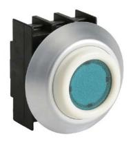
Schmersal pushbutton, IP67 and IP69K, 22mm, momentary, operator only, plastic base, plastic bezel, Operator: green, extended, 27mm, round, plastic. Requires contact and light blocks.
