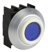
Schmersal pushbutton, IP67 and IP69K, 22mm, momentary, operator only, plastic base, plastic bezel, Operator: blue, extended, 27mm, round, plastic. Requires contact and light blocks.
